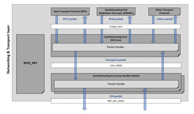
Figure 22: GeoNetworking packet handling
