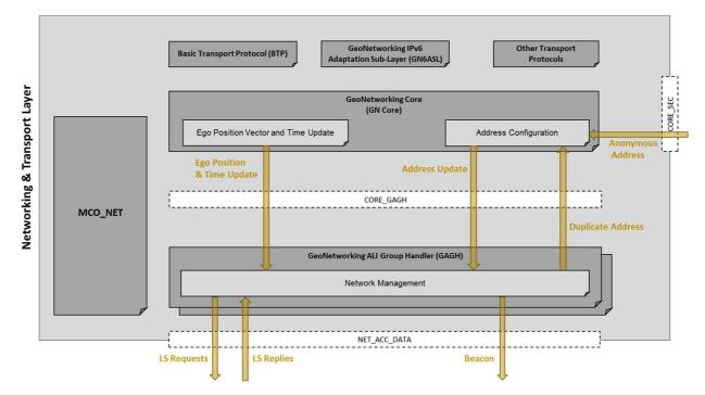
Figure 20: Overview of Network Management functions and control flow
