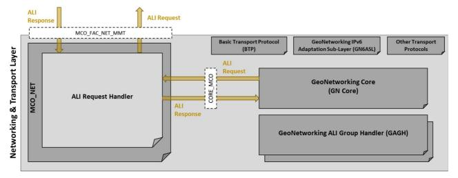
Figure 26: Handling of packet with no assigned ALI
